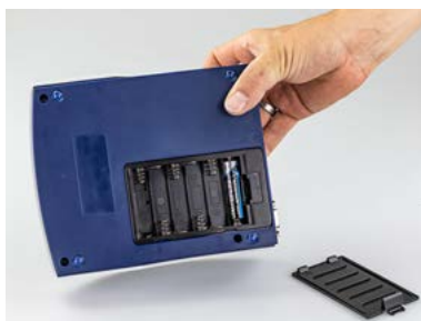
Pic. 11: Battery compartment
